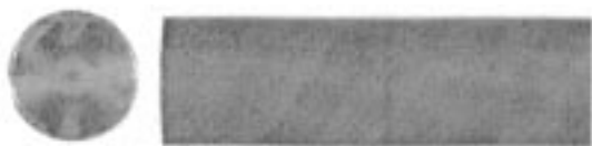
FIG. 1 Acceptable View of the Break Face.
